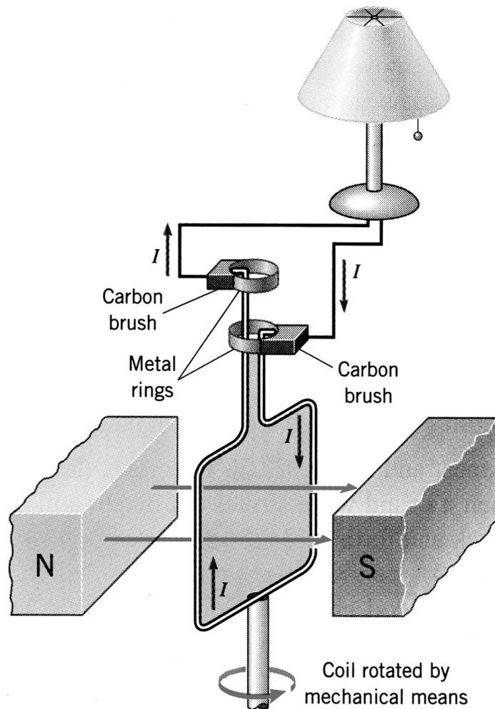
Although not shown in the diagram, the wire is usually wound around an iron core. The coil/core combination is called the **armature**. Each end of the wire forming the coil is connected to the external circuit by means of a metal ring that rotates with the coil. Each ring slides against a stationary carbon brush, to which the external circuit is connected.
