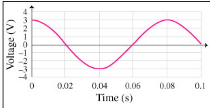
The result of this is that, for half of the rotation, the current in the loop flows clockwise, while for the other half it flows counterclockwise. This is referred to as **alternating current** or simply **AC**.
